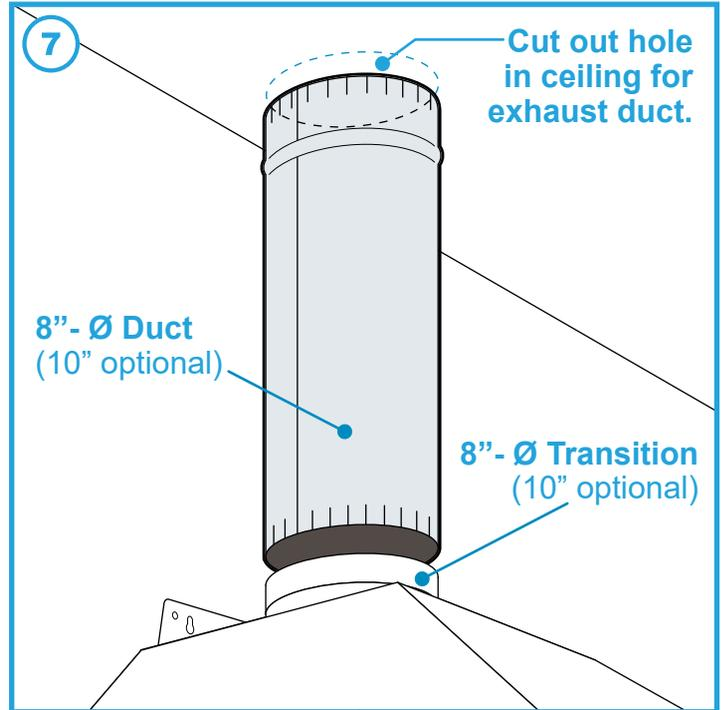
Use 8" round steel pipe (follow building codes in your area) to connect the exhaust on the hood to the ductwork above. Use aluminum tape to make all joints secure and air tight.
