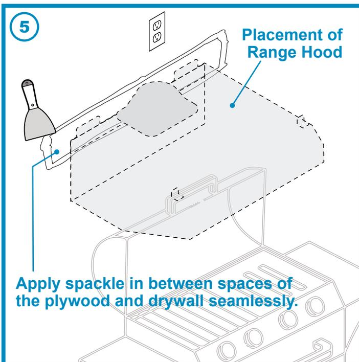
(5) Apply spackle in between spaces of the plywood and drywall seamlessly. Sand down any rough spackle to smooth out.
