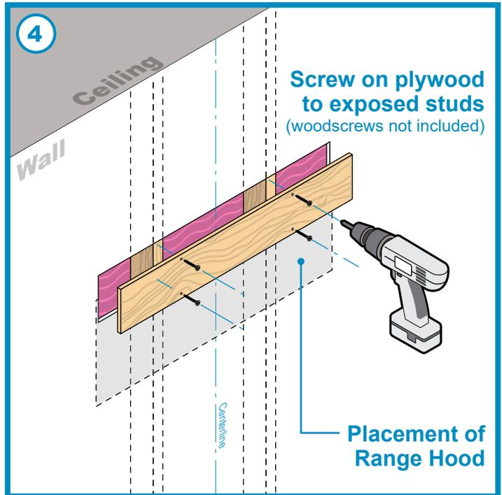
(4) Fasten #8 2-1/2" woodscrews (not included) to mount onto the plywood based on your earlier measurements already established.
