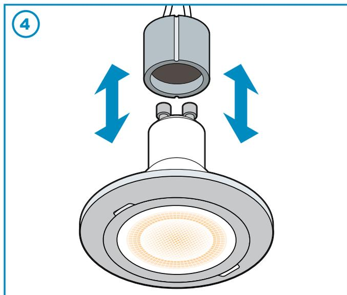
**(3)** Twist the connector cap off, and **(4)** dislodge from electrical tether. LED Bulb is model: **GU10**. Contact Victory Range Hood and place an order, or you may purchase at your nearest hardware store.
