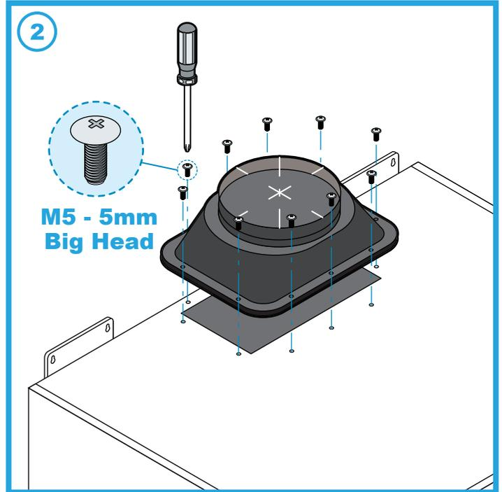
(2) Screw on 8" - Ø Transition on to the top exhaust of range hood (10" Optional).
