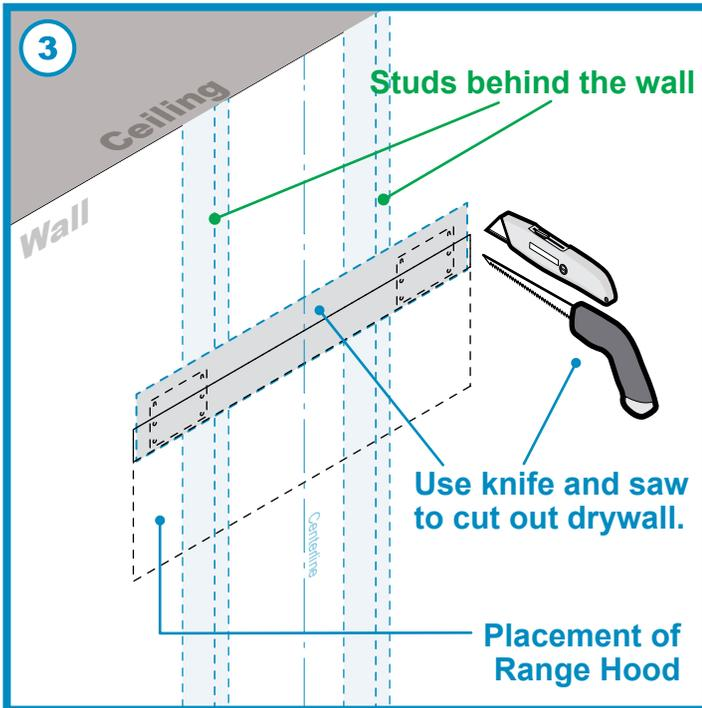
(3) Use knife and saw to cut out drywall to accommodate plywood brace support. The inserted plywood should be the same depth as the drywall slab it is replacing.
