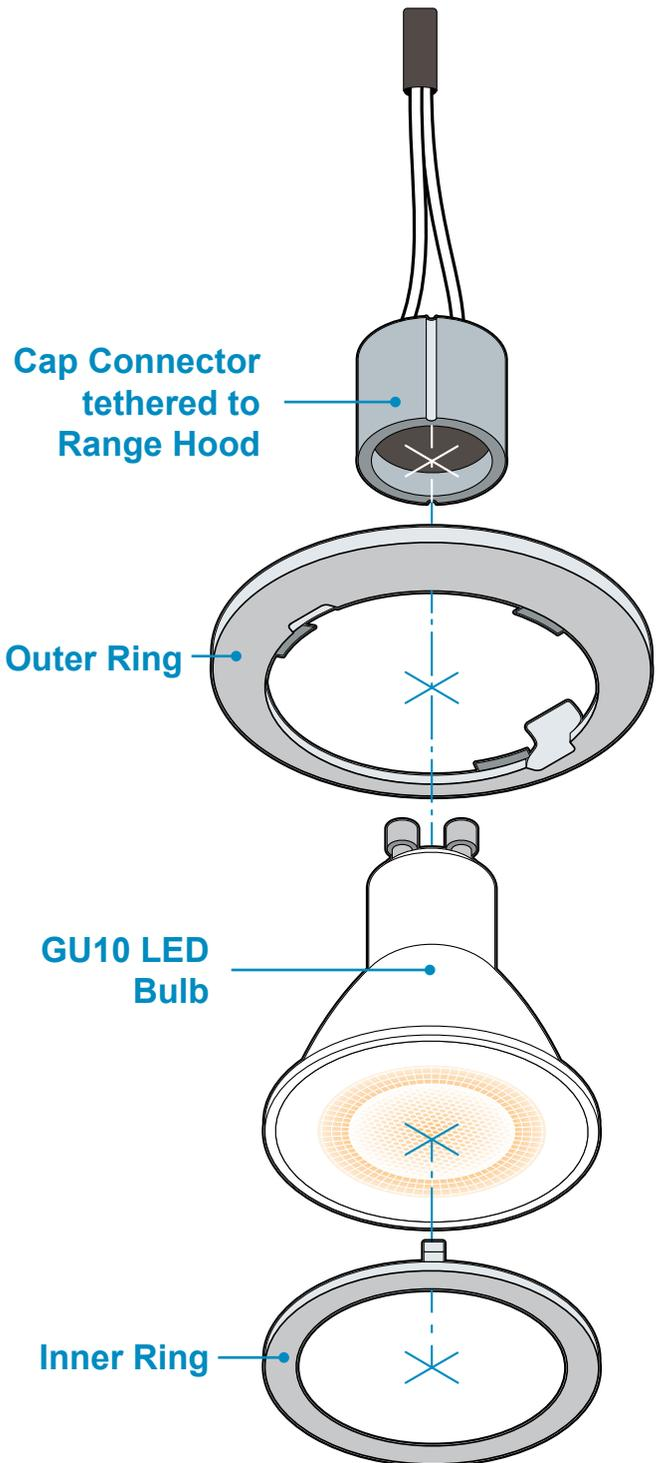
To re-assemble, simply reverse the steps **(6)** to **(2)**. To re-install, **(7)** press the bulb housing carefully and firmly into the recess, until you hear a positive snap.
